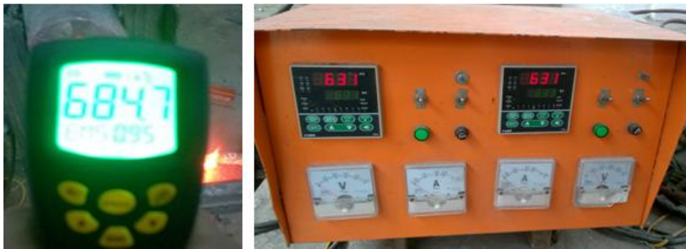
Fig.3 Resistance heat output device and measuring device, temperature monitor
