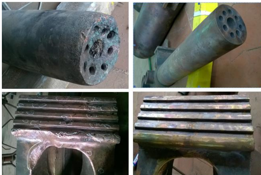
Fig.5 Details before and after welding recovery
